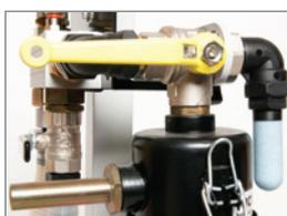
**Clamping valve kit** Harness the powerful but gentle holding power of vacuum, by adding the clamping valve kit to the Vacmobile 20/2. This accessory is ideal for vacuum holding applications during routing or surface finishing, as vacuum clamping does not mark the top side and allows 100% access to the part perimeter. The kit includes a quick changeover valve (to allow instant release of the part being held) and a reverse flushed dust filter.
